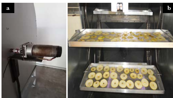
Figure 3. Rotation system. (a) Coupled geared motor. (b) Tray distribution.
