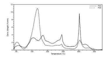
Figure 6. TGA curve of orange peel bioplastic films.
