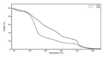
Figure 5. TGA curve of orange peel bioplastic films.
