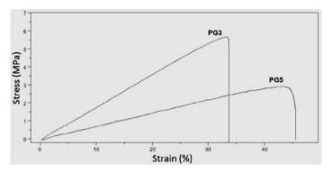
Figure 3. Stress-strain curve of bioplastic films.
