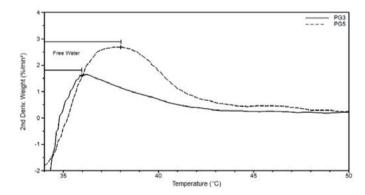
Figure 7. 2ndDTG curve (second derivative of thermal degradation) corresponding to water loss in PG3 AND PG5 samples.
