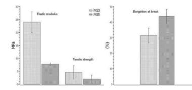
**Figure 4**. Mechanical properties of bioplastic film. The bars indicate the standard deviation. In all parameters, the proportion of glycerol produced changes with statistical significance p<0.05.
