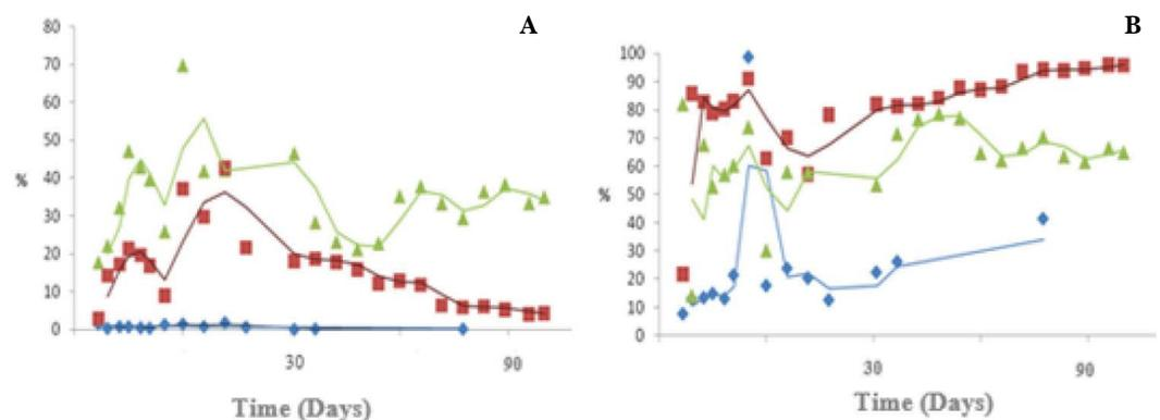
**Figure 1.** Percentage of (A) methane and B) CO<sub>2</sub> from anaerobic digestion BM, bovine manure (■), RST (residual sludge from tilapia fish Breeding ponds) (◆), and BMMR mixture 1:1 BM-RST (▲). Data are the mean of seven jars×three experiments×three measurements by each day of collection. Whole experiment lasted 90 days.
