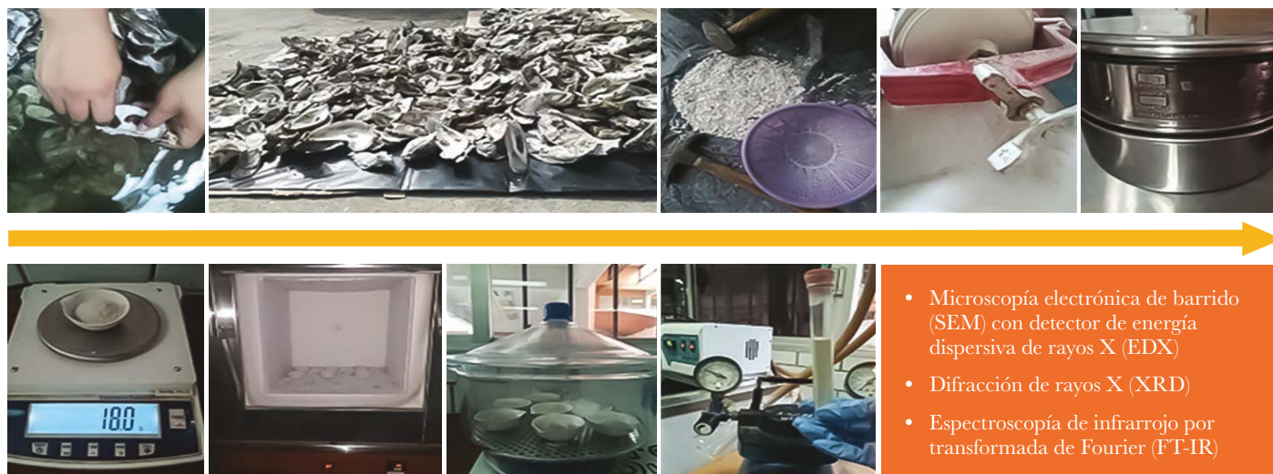
Figure 1. Preparation of CaO catalyst derived from oyster shells.
