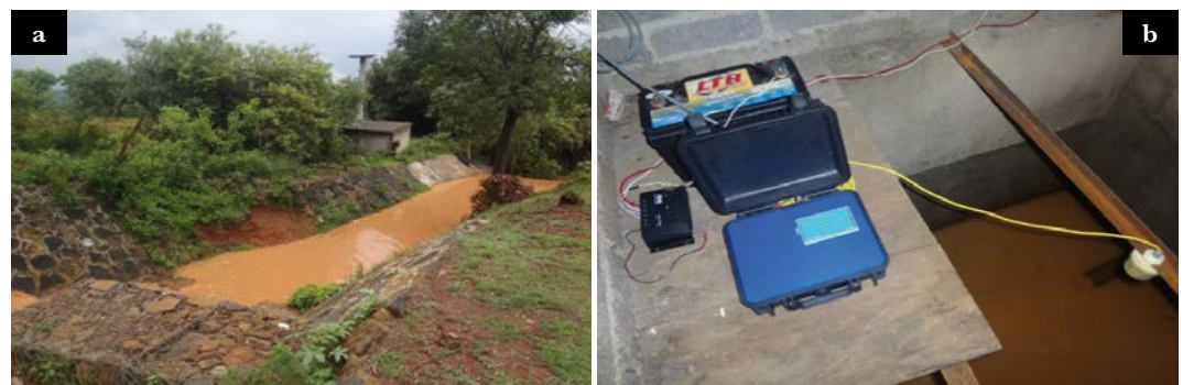
Figure 2. long-throat gauge (a) and ultrasonic sensor equipment (b) used to record the runoffs.
