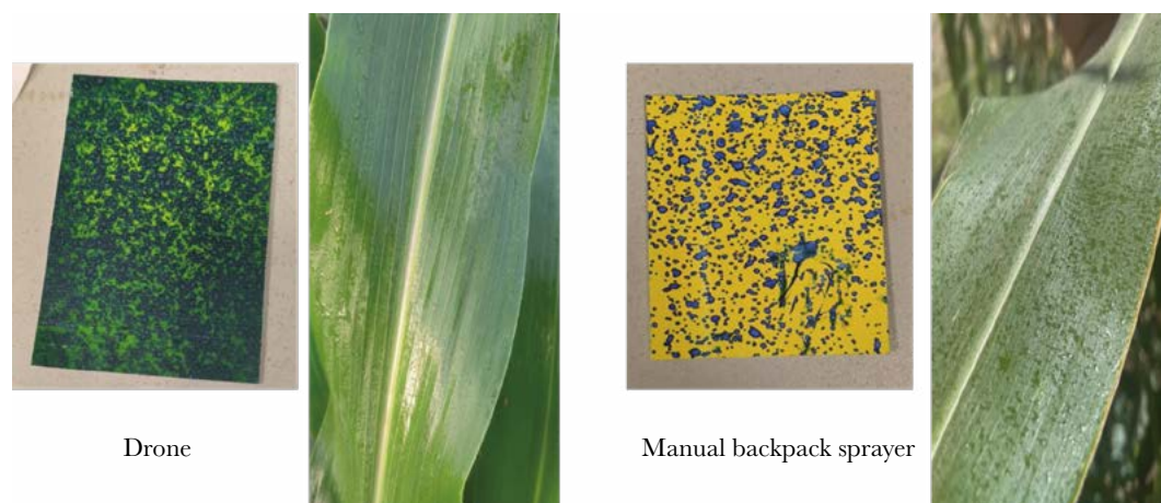
Figure 2. Comparative assessment of water-sensitive cards and foliage following foliar applications with both application methods.
